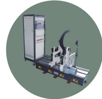
Dynamic balance inspection of spindle motor
